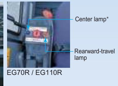
EG70R / EG110R Center lamp* Rearward-travel lamp * Lit when the upper structure and undercarriage become paralleled.
