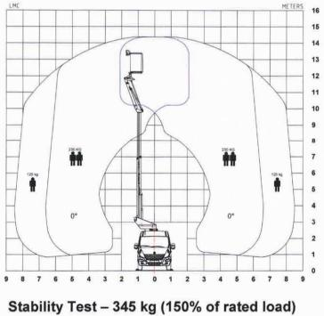
Slope – 3.5° transverse, 5.5° longitudinally Overload Test – 288 kg (125 % of rated load)
